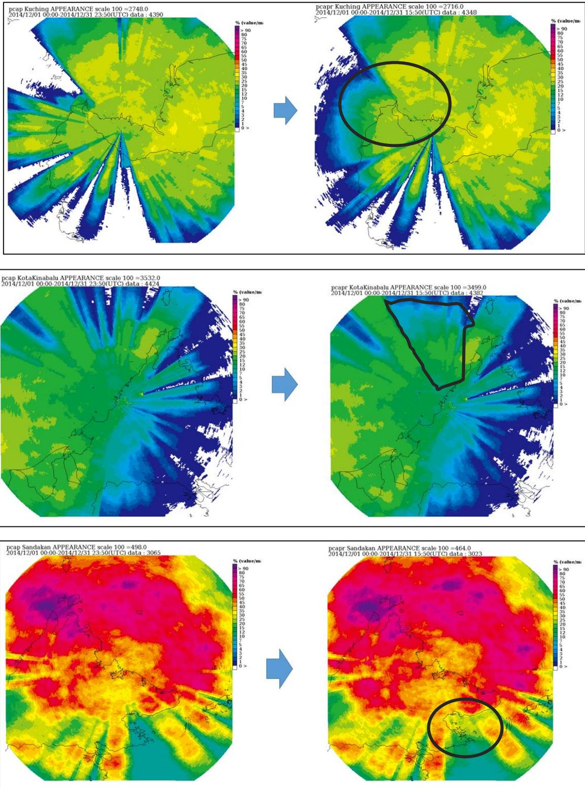
Figure 30: The modification and adjustment of EIL table for each radar stations are performed to gain better coverage and intensity
