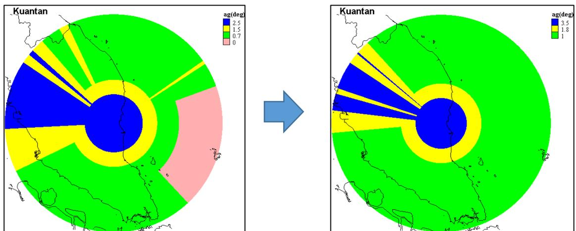
Figure 4: The performance of radar observation for each elevation angles and its improvement of new elevation angles
