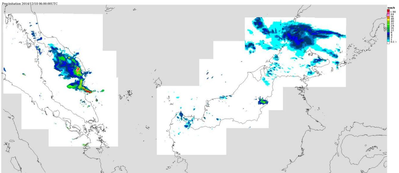
Figure 35: The composite of radar images after QPE calibration with raingauges
