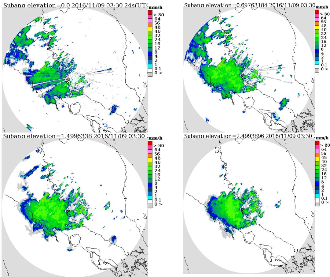
Figure 7: The performance of radar observation for each elevation angles
