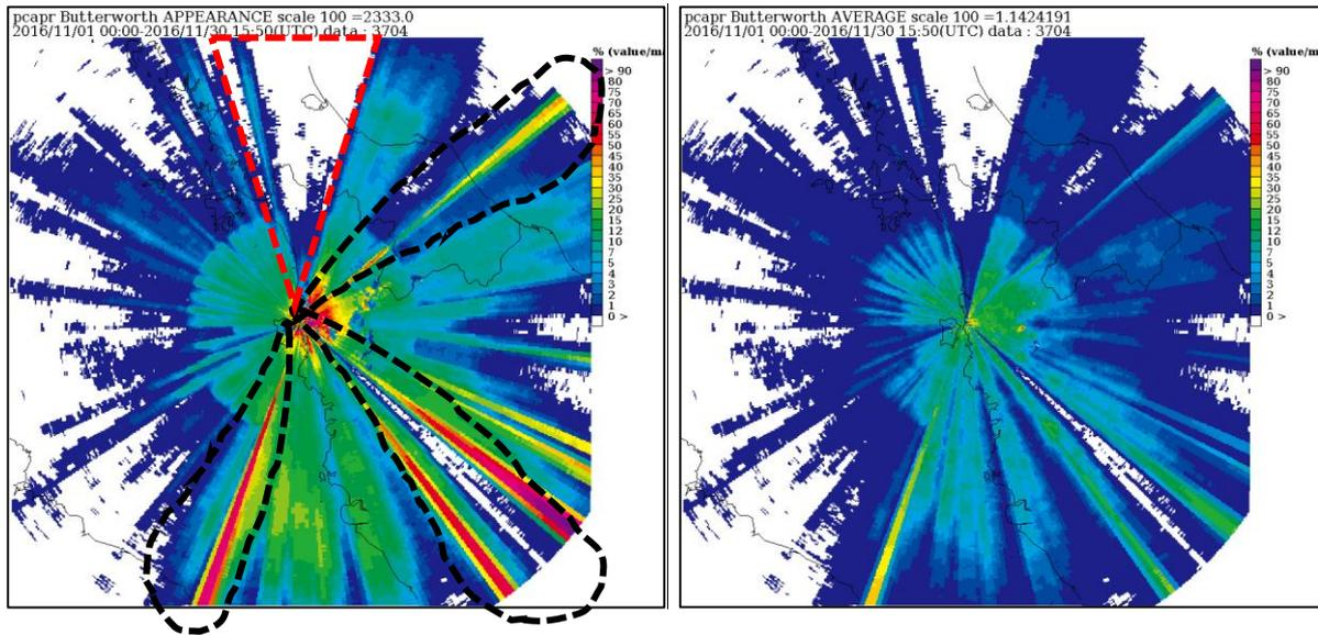
Referring to Table 1, the appearance data value is high meanwhile the average data showed lower value. This images indicate BW1 has suspicious data with clutter caught is weak but continuous indicator for interference problems (black dashed line). From these statistical images from 01 Nov-30 Nov 2016, described the blockage areas as shown in red color dashed line.
