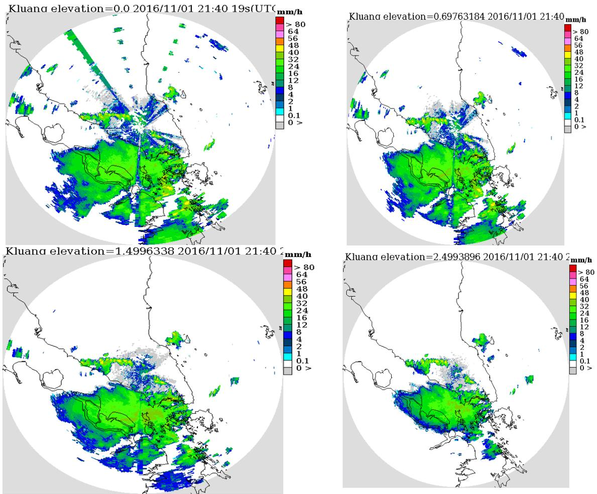
Figure 5: The performance of radar observation for each elevation angles
