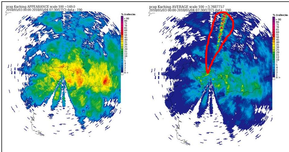
Figure 23: PCAPPI statistical data to show the interference signal
