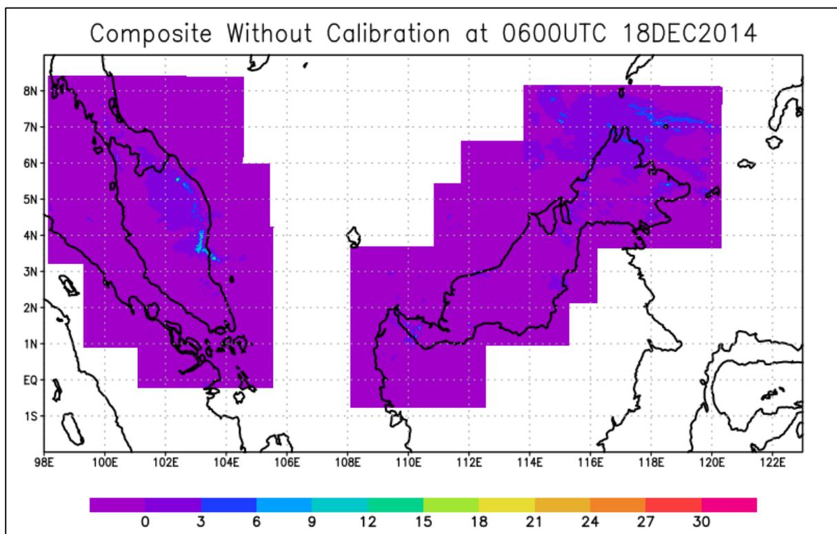
Figure 32: The non-calibration QPE composite radar indicated the underestimation of radar rainfall
