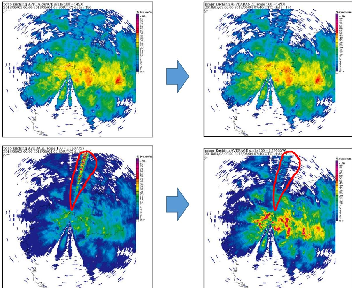
Figure 26: The comparison before and after the EIL modification resulting in the elimination of interference on the radar images
