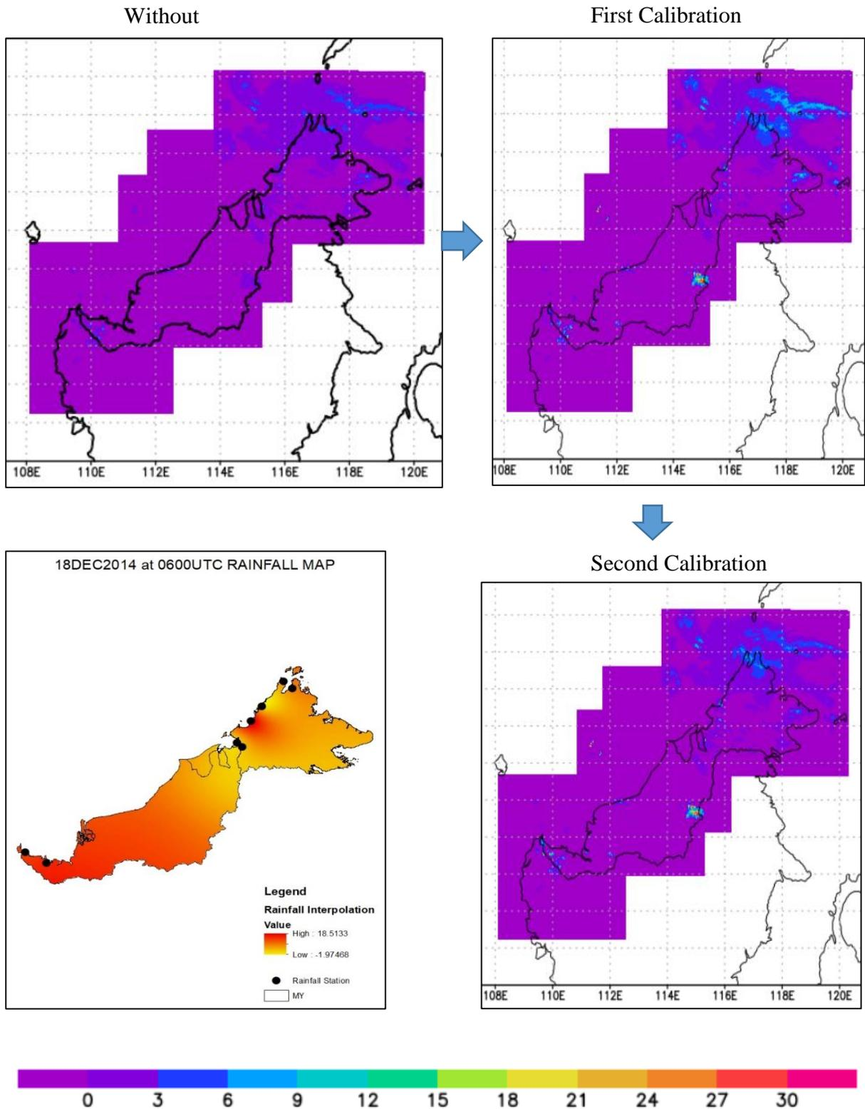
Figure 37: The comparison before and after the calibration with raingauges by using only 8 good stations
