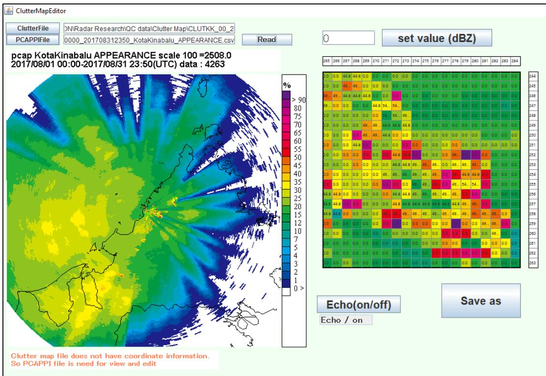
Figure 28: Clutter map software to remove the clutter for KK1 radar station
