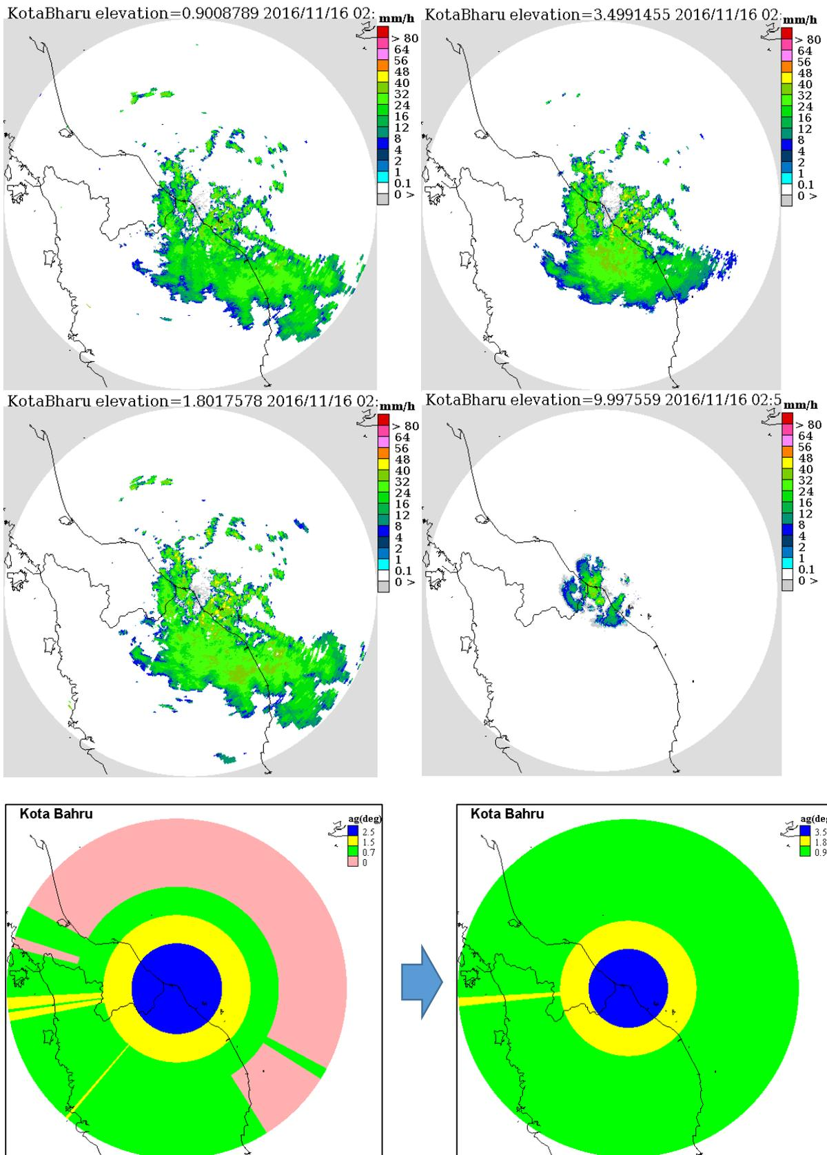
Figure 2: The performance of radar observation for each elevation angles and its improvement of new elevation angles
