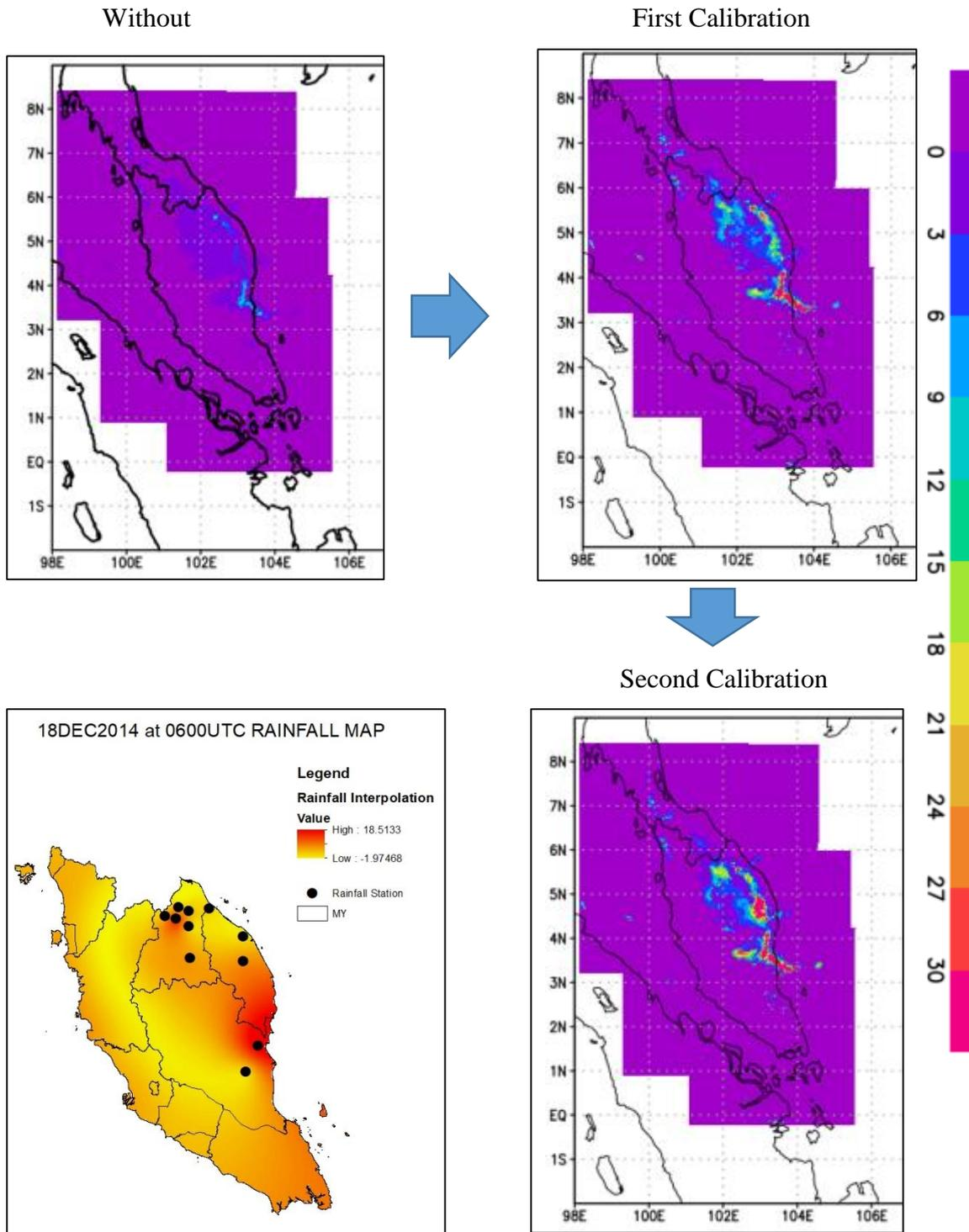
Figure 36: The comparison before and after the calibration with raingauges by using only 11 good stations
