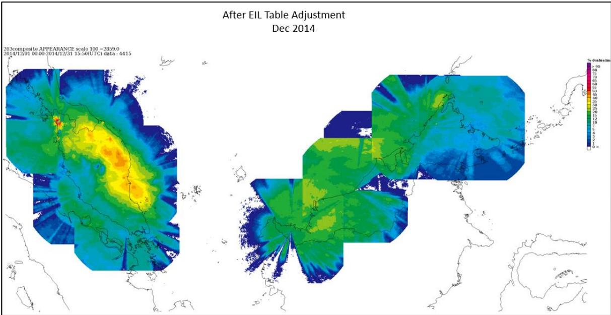
Figure 31: The statistical performance data in December 2014 after applying the technique of EIL Table adjustment
