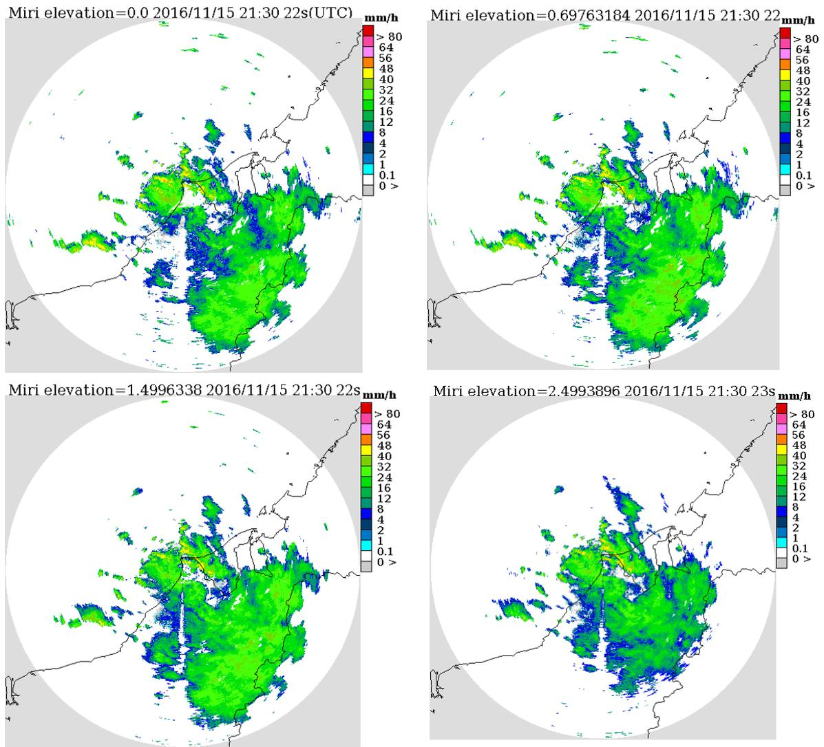
Figure 17: The performance of radar observation for each elevation angles
