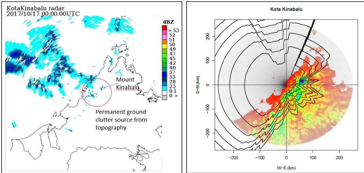
Figure 27: The ground clutter source from Mount Kinabalu data existed on the KK1 radar image
