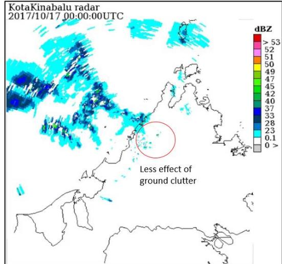
Figure 29: The comparison before and after using clutter map
